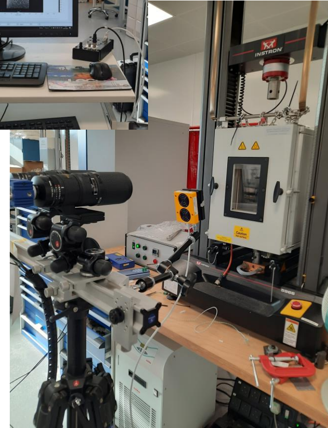
Stereo digital image correlation (DIC) setup gathering thermal stress data from the simple monoblock model.
