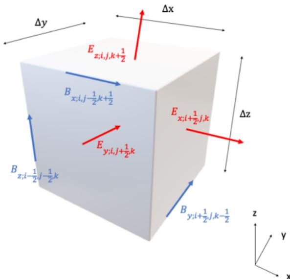
**Figure:** Collocation of the electromagnetic fields in FDTD. The magnetic field is defined at the edges and the electric field is defined at the faces.
