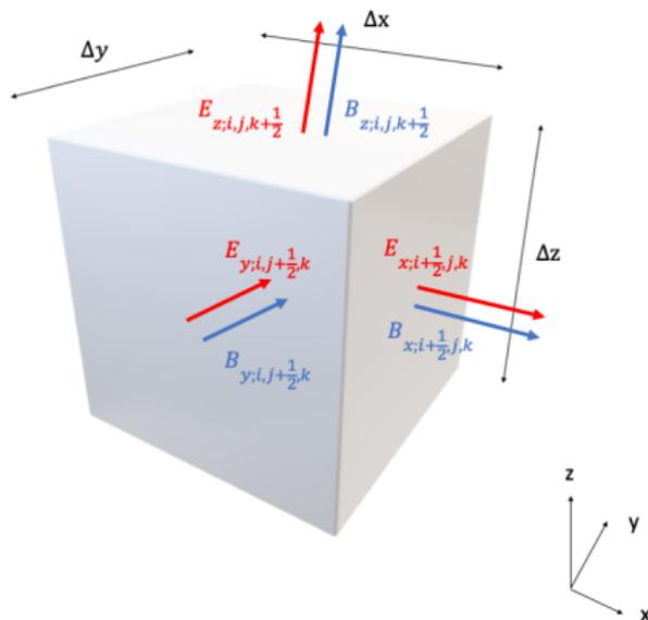
**Figure:** Collocation of the electromagnetic fields in FVTD. The magnetic field and the electric field are defined at the faces.
