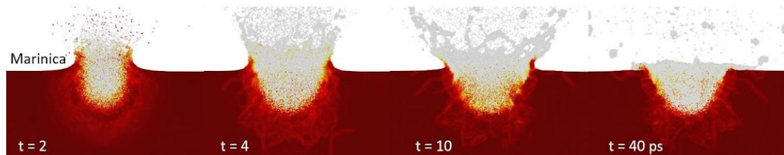
Figure 1: MD Simulation of 8 nm W spherical dust Impacting on W Single-Crystal Target at 3 km/s: Time Evolution at 2, 4, 10 and 100 ps.
